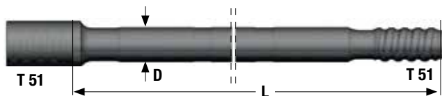
Flushing hole \varnothing 21.5 mm. Female end \varnothing 71 mm
